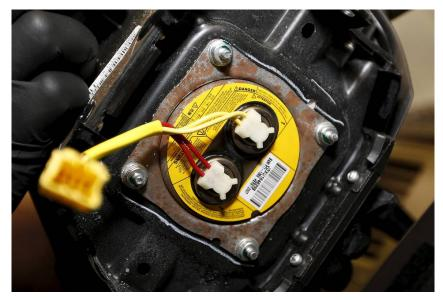
A recalled Takata air bag inflater. The Japanese company agreed to phase out its use of a suspect chemical by 2018. PHOTO: ASSOCIATED PRESS
